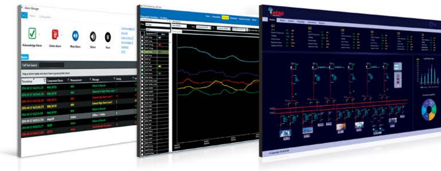
Electrical SCADA Human Machine Interface templates
